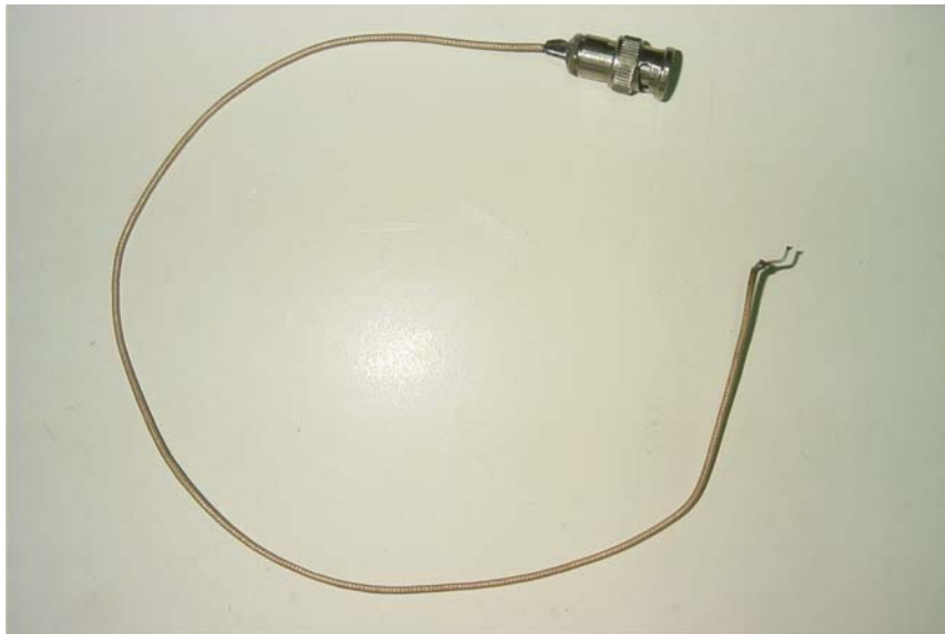
Figure 2.2. RF test cable
