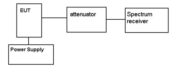
**METHOD OF MEASUREMENT:** The procedure used was TIA/EIA-603 Standard without any exceptions. The measurements were made at TIMCO ENGINEERING INC. 849 N.W. State Road 45, Newberry, Florida 32669.
