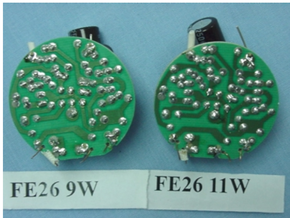
Figure 6 Energy Saving Lamp (M/N: FE26 9W, FE26 11W) SOLDERED SIDE
