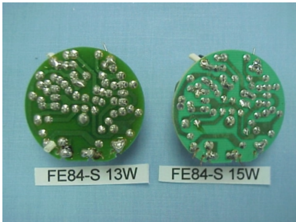
Figure 18 Energy Saving Lamp (M/N: FE84-S 13W, FE84-S 15W) SOLDERED SIDE
