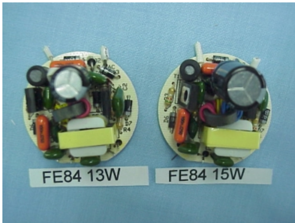
Figure 27 Energy Saving Lamp(M/N: FE84 13W, FE84 15W) SOLDERED SIDE
