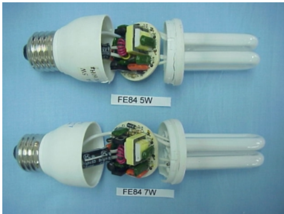
Figure 19 Energy Saving Lamp(M/N: FE84 5W, FE84 7W) COVER REMOVED
