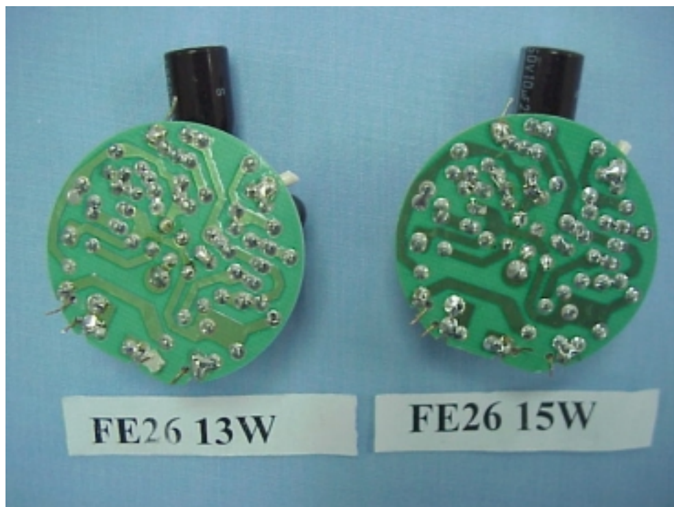
FIGURE 9 ENERGY SAVING LAMP (M/N: FE26 13W, FE26 15W) SOLDERED SIDE
