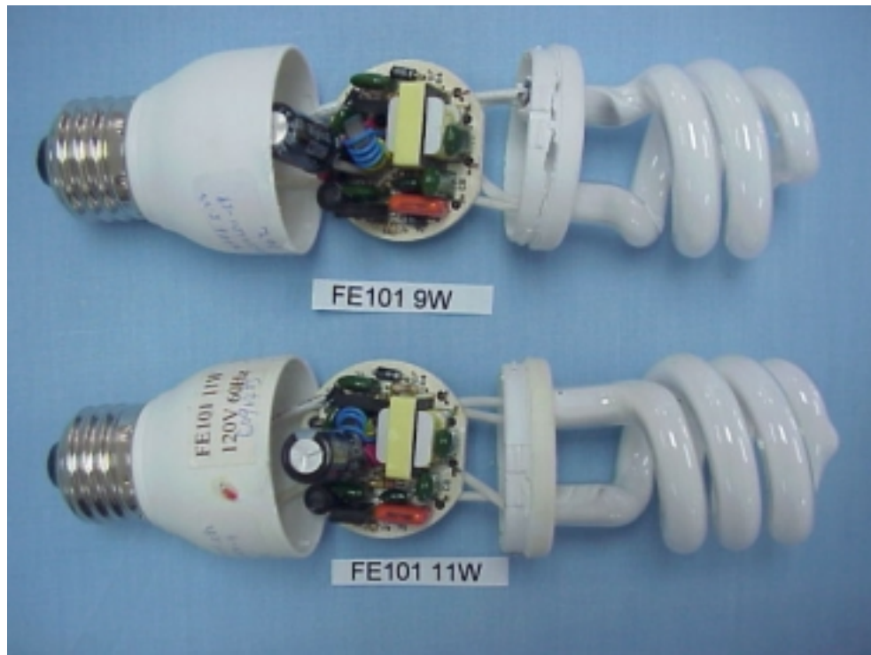
Figure 31 Energy Saving Lamp(M/N: FE101 9W, FE101 11W) COVER REMOVED
