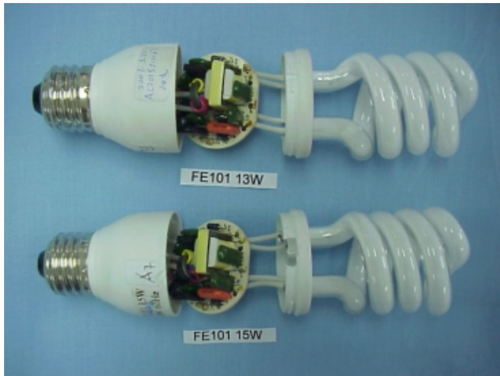
Figure 34 Energy Saving Lamp(M/N: FE101 13W, FE101 15W) COVER REMOVED
