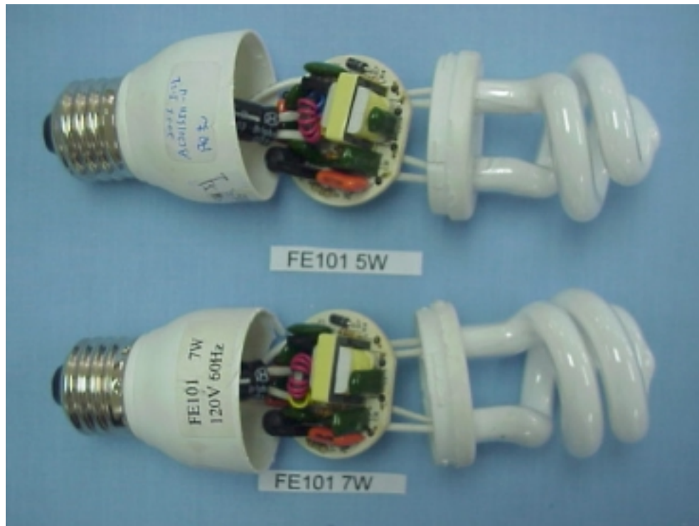
Figure 28 Energy Saving Lamp(M/N: FE101 5W, FE101 7W) COVER REMOVED
