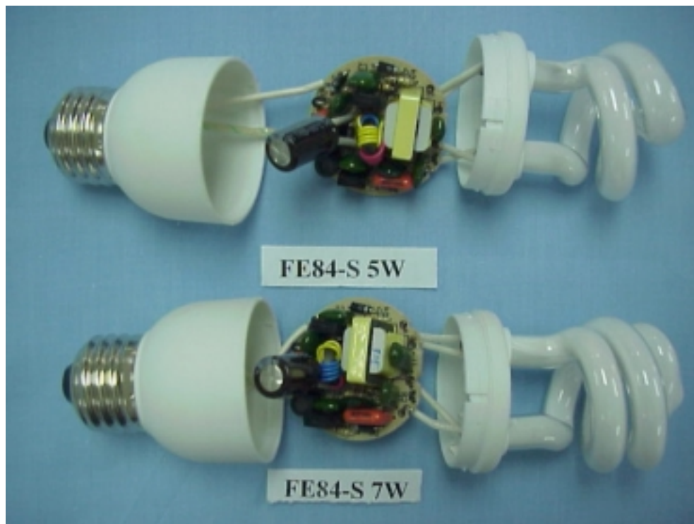
Figure 10 Energy Saving Lamp (M/N: FE84-S 5W, FE84-S 7W) COVER REMOVED
