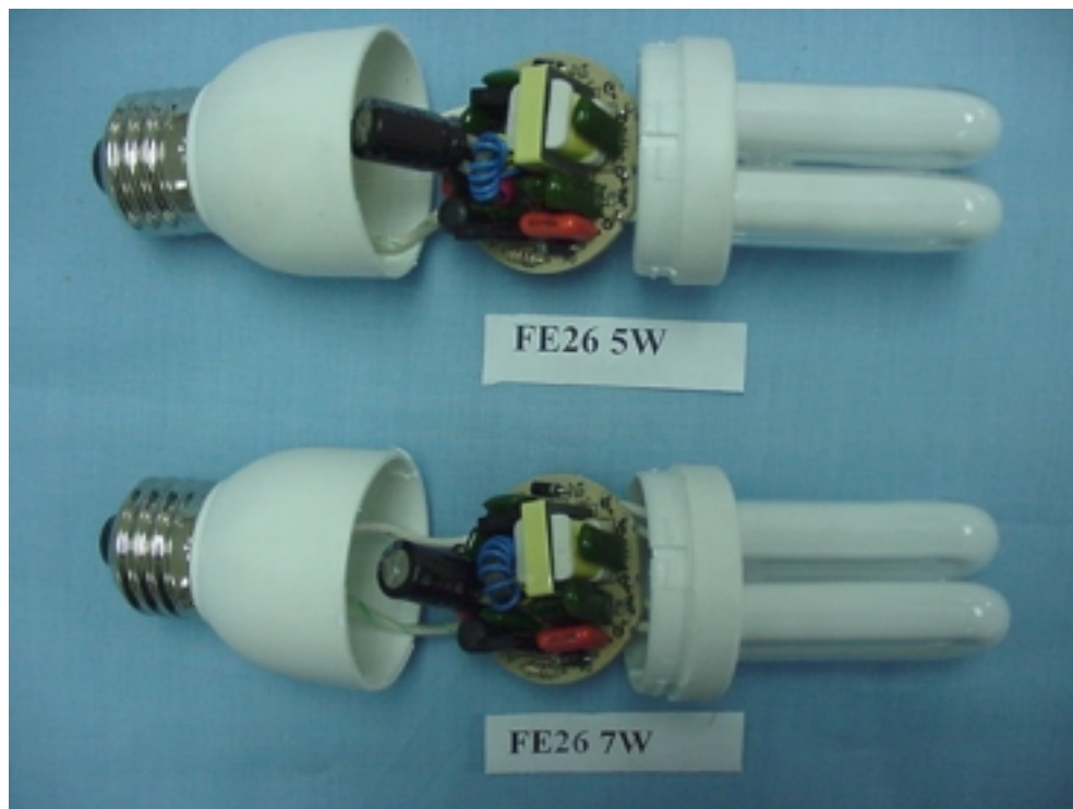
Figure 1 Energy Saving Lamp (M/N: FE26 5W, FE26 7W) COVER REMOVED
