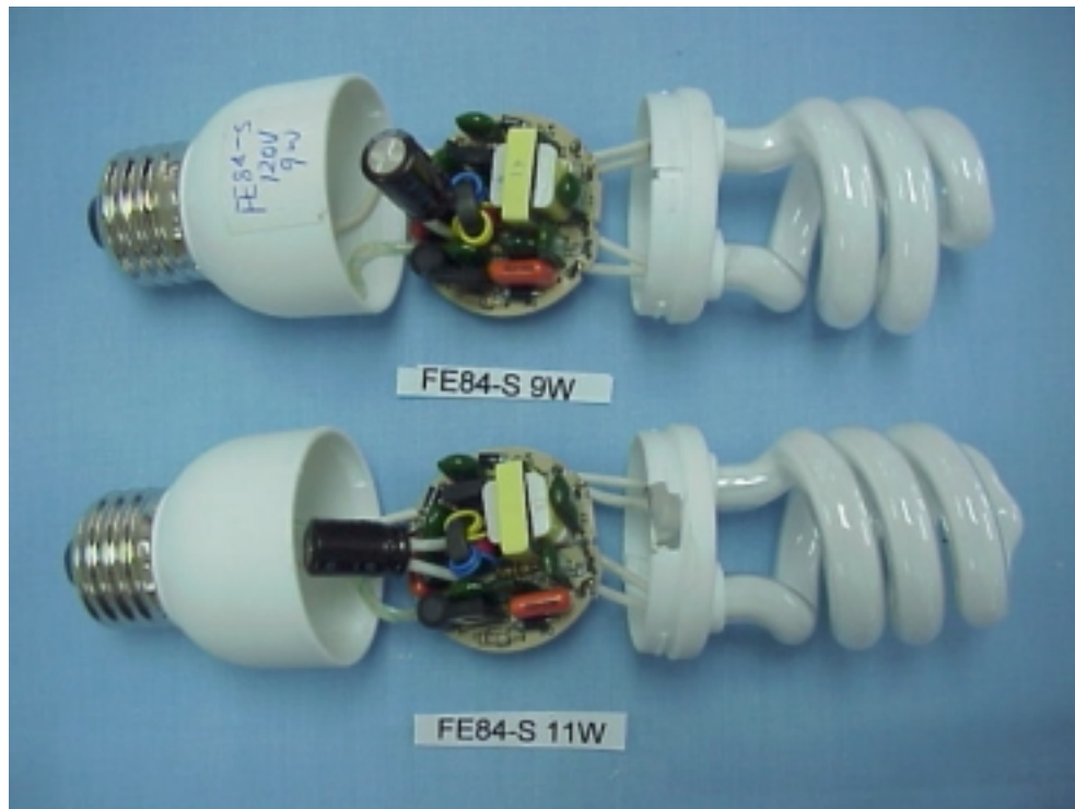
Figure 13 Energy Saving Lamp (M/N: FE84-S 9W, FE84-S 11W) COVER REMOVED
