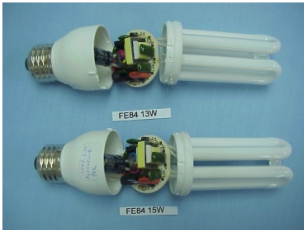
Figure 25 Energy Saving Lamp(M/N: FE84 13W, FE84 15W) COVER REMOVED
