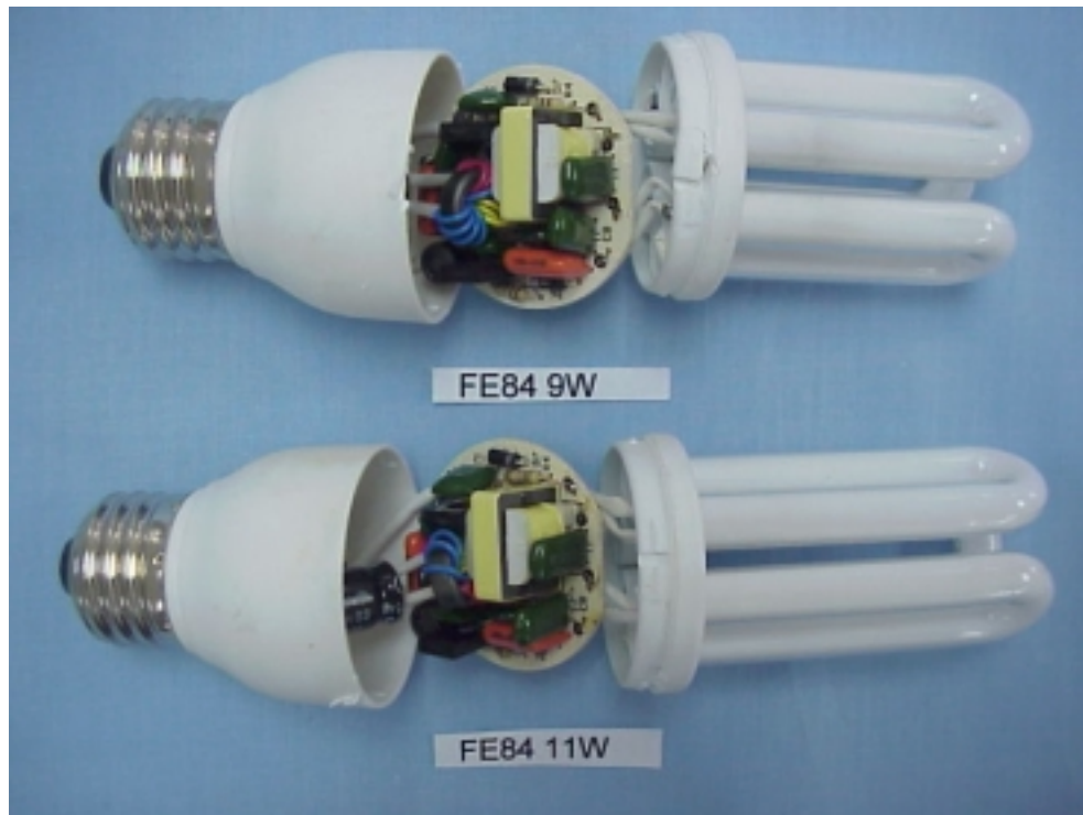
Figure 22 Energy Saving Lamp(M/N: FE84 9W, FE84 11W) COVER REMOVED
