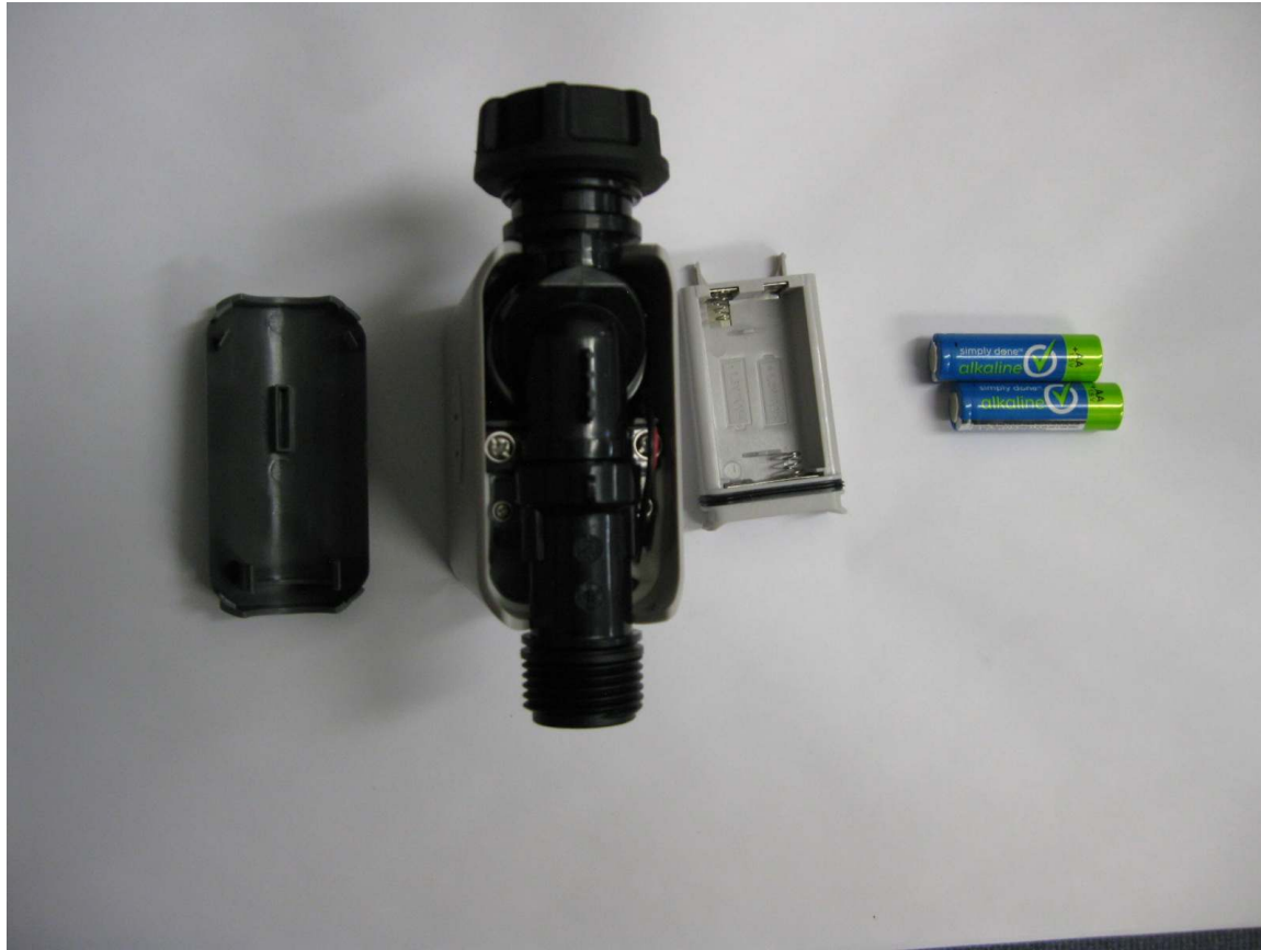
Figure 1 - Access cover removed and battery compartment removed.
