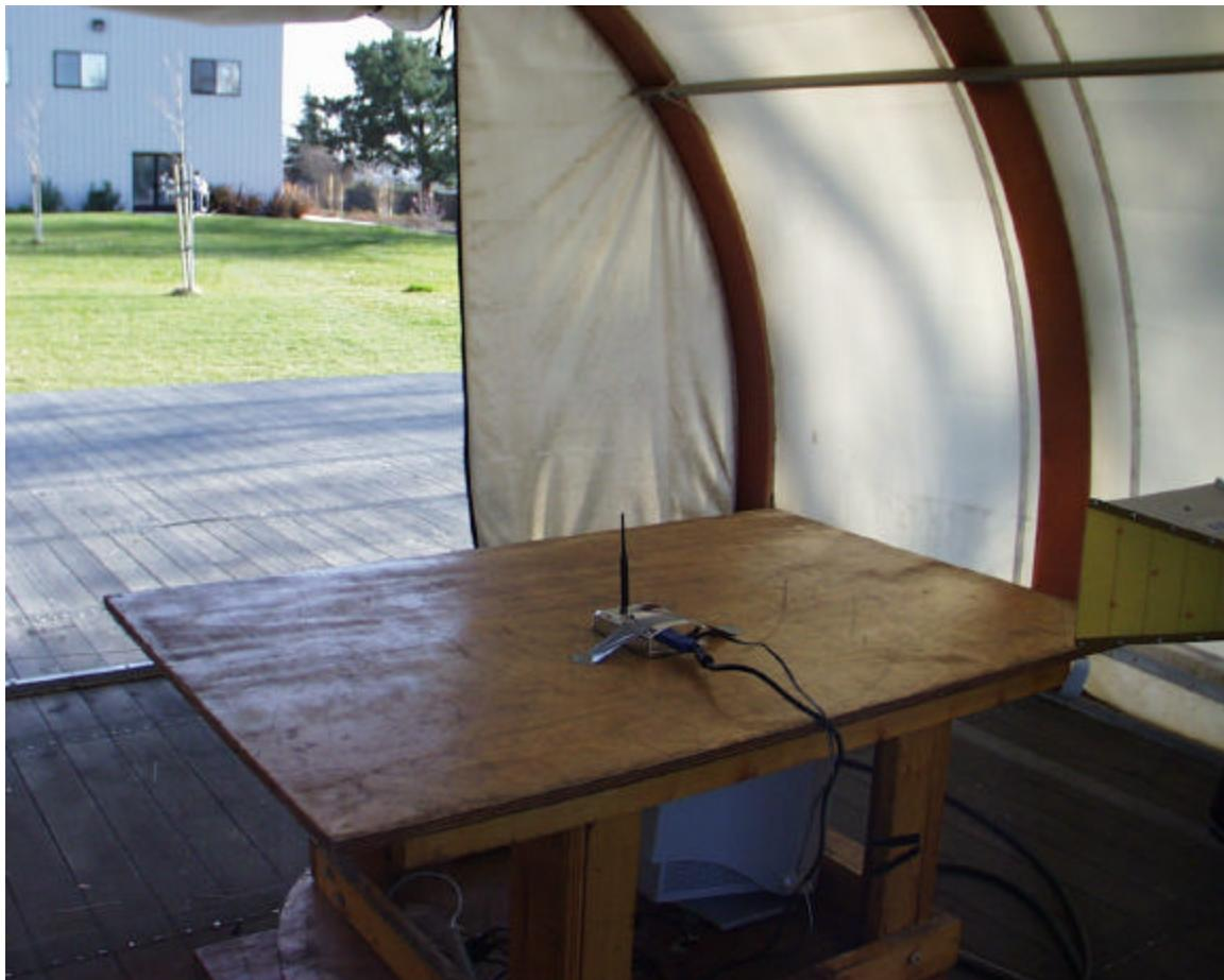
**DIGITAL DEVICE RADIATED EMISSIONS MEASUREMENT SETUP**
