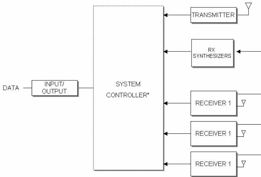
\*System Controller houses modem, diversity, Ethernet, and transmit processing
