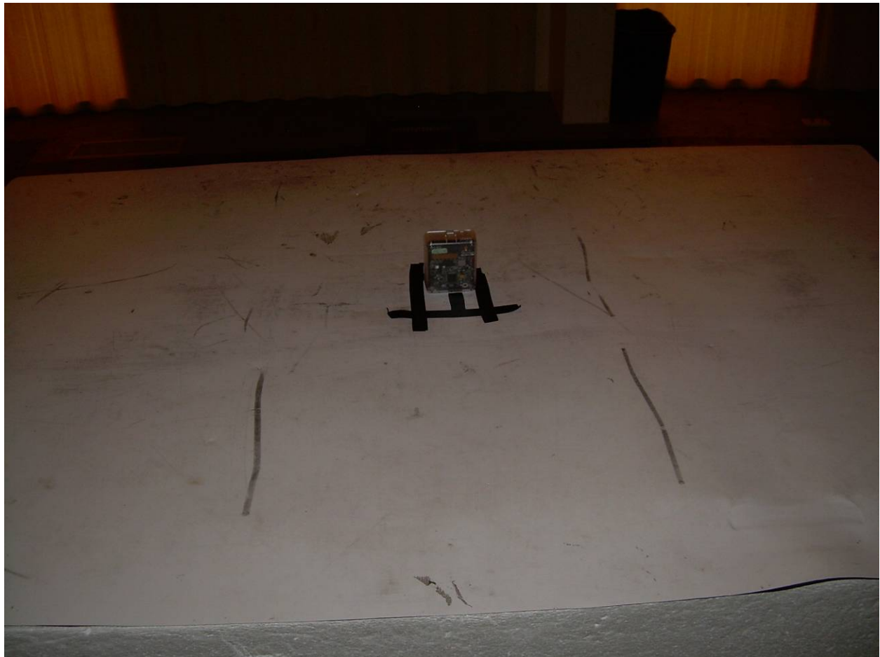
Photograph 2 – View Radiated Disturbance – Vertical, Internal Antenna Configuration
