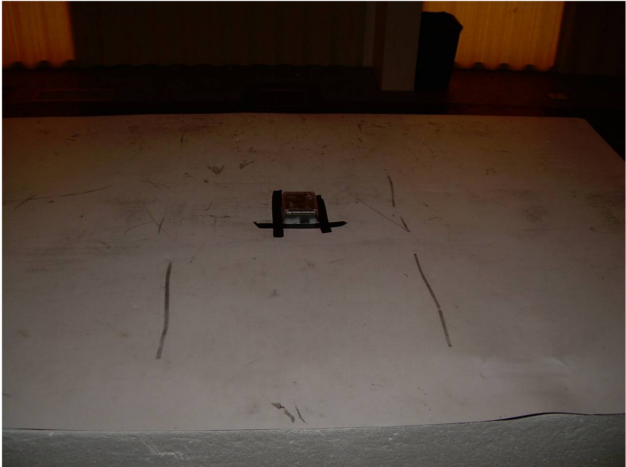
Photograph 1 – View Radiated Disturbance Worst Case Configuration – Horizontal, Internal Antenna
