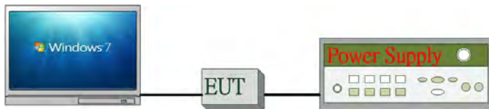
Fig. 2-1 Conducted (Antenna Port) Emission Configuration
