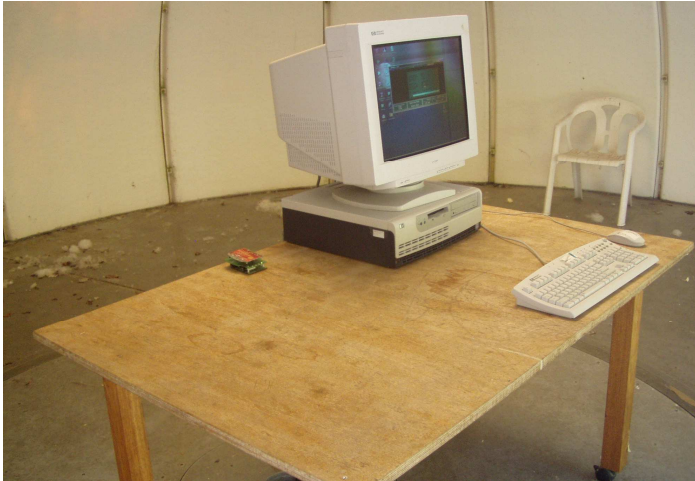
Radiated emission test setup
