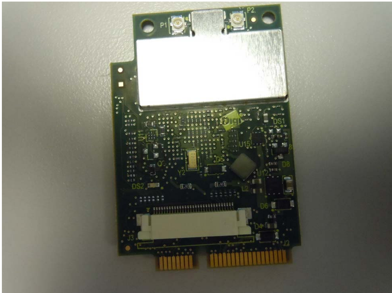
ConnectCard for i.MX28 With two RF Ports-- Top View
