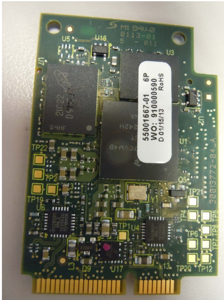
ConnectCard for i.MX28 With One RF Ports-- Bottom View
