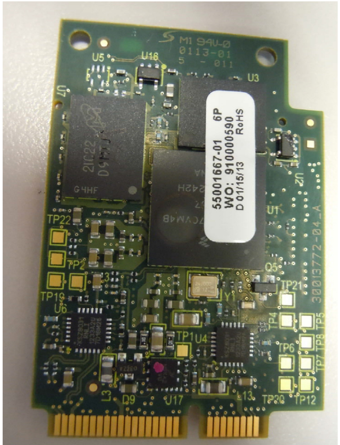
ConnectCard for i.MX28 With One RF Ports-- Bottom View
