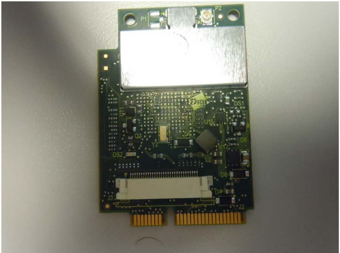
ConnectCard for i.MX28 With One RF Port-- Top View
