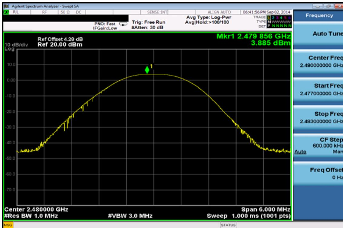
Peak Power Output Data Plot (CH Low) (EDR mode  $\pi/4$ DQPSK)
