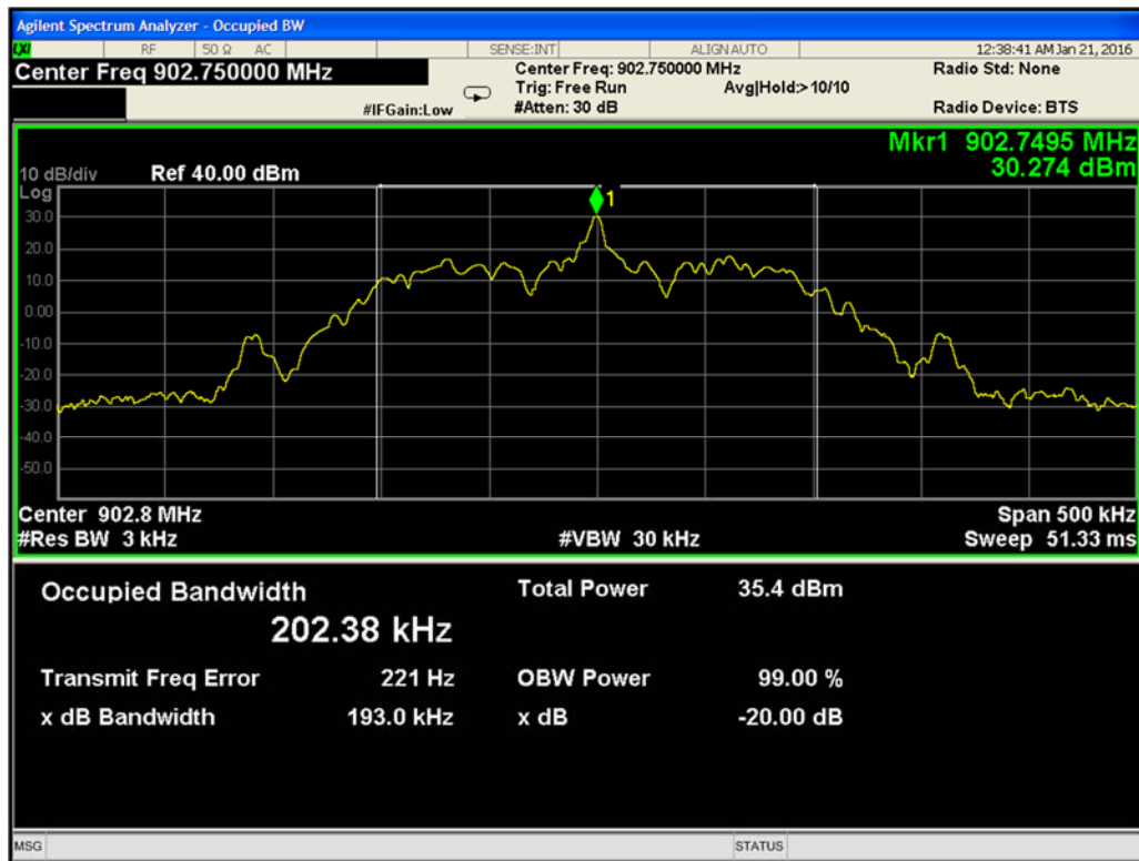
Occupied Bandwidth – FCC Part 15.247 Low Channel/High Data Rate
