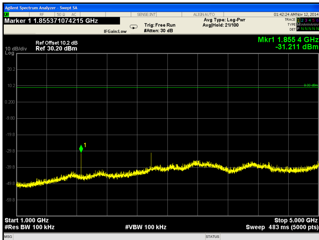
Conducted Spurious Emissions High channel
