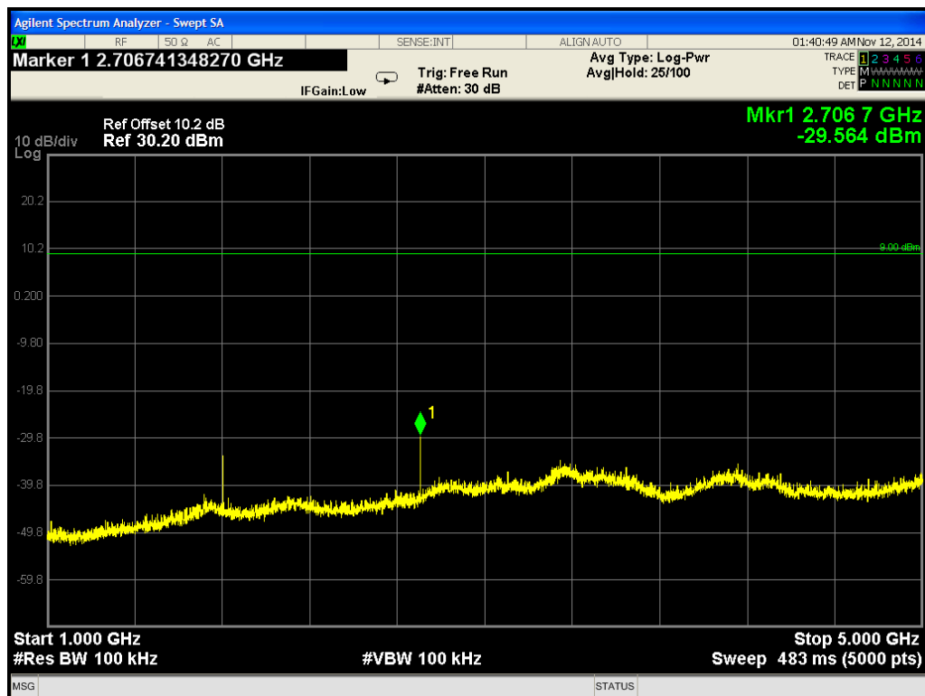
Conducted Spurious Emissions Low channel
