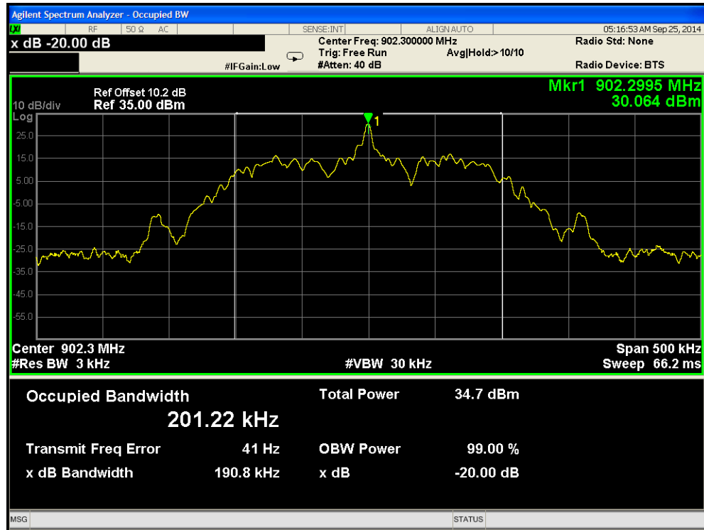
Occupied Bandwidth – Dense Mode Low (higher data rate)
