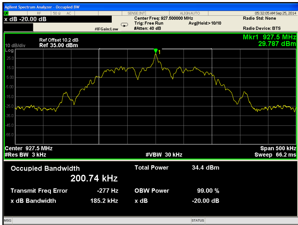
Occupied Bandwidth – Dense Mode High (higher data rate)
