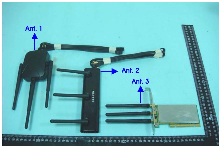
Note: The EUT has three sets of dipole antenna.
