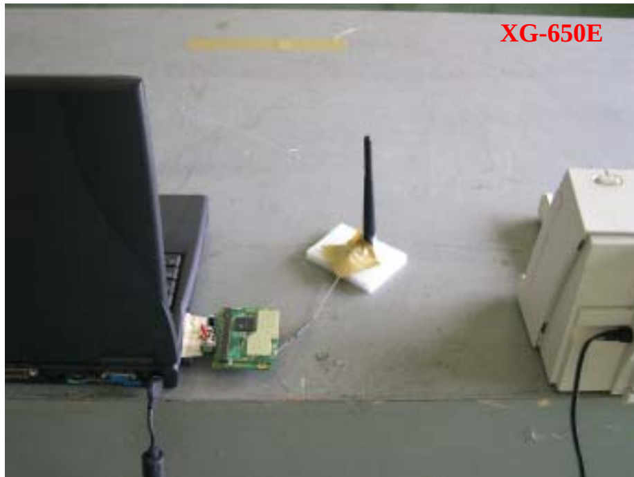
Photo 3: Radiated Emission Test Set-up
