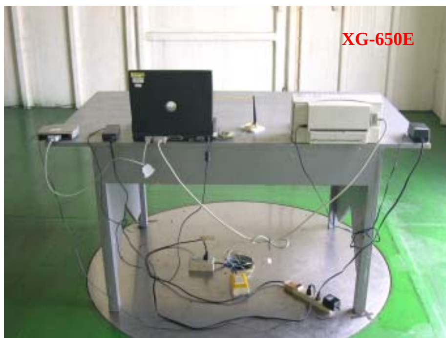
Photo 2: Radiated Emission Test Set-up
