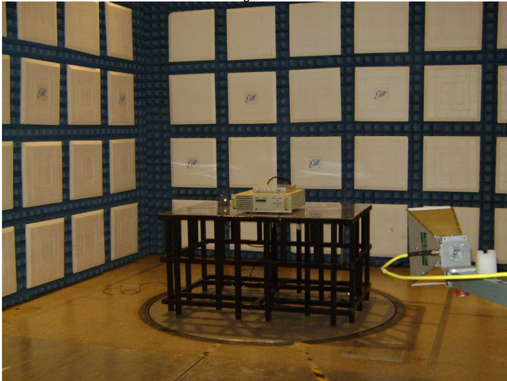
Test Set-up for Radiated Emissions, 1GHz to 2.5GHz – Horizontal Polarization
