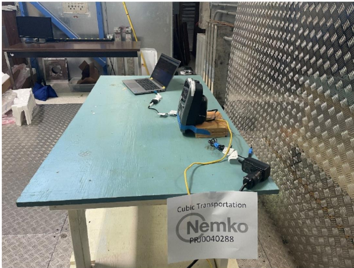
Figure 8.2.2 Conducted disturbance at AC mains port setup photo (Back)
