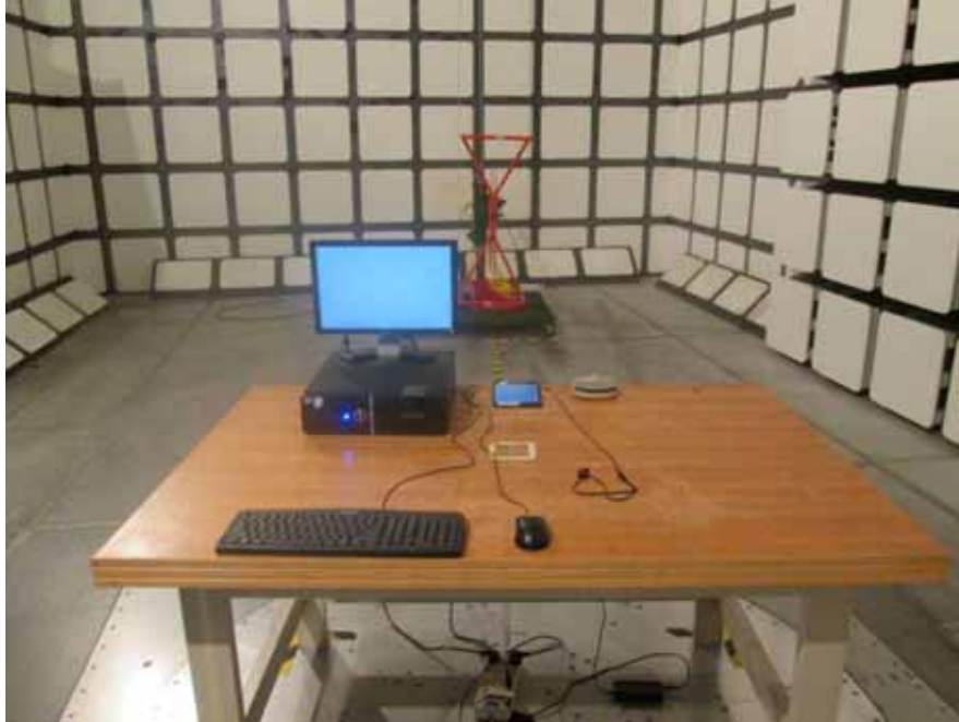
Radiated Emissions – Front View (Below 1 GHz)
