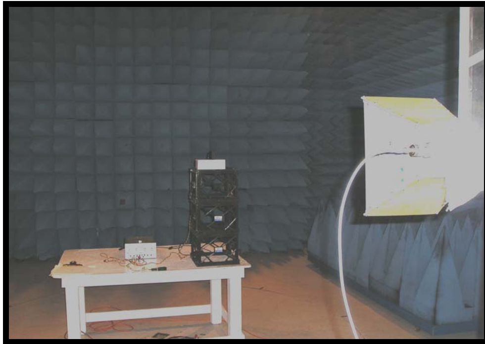
Figure 9: Spurious emissions above 1 GHz (front view)
