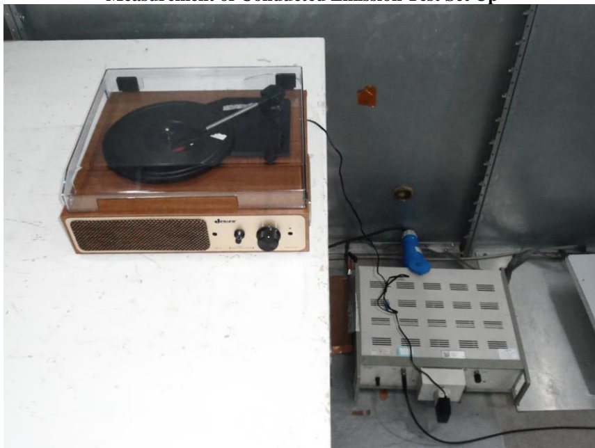
Measurement of Conducted Emission Test Set Up
