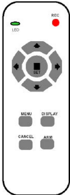
**REC** : Recording, record current image when this button is push down.
