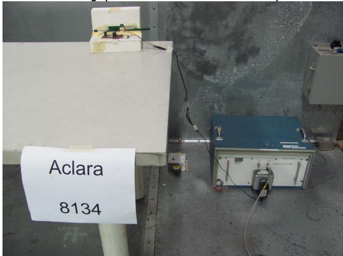
Photographs of Conducted Emissions Test Setup
