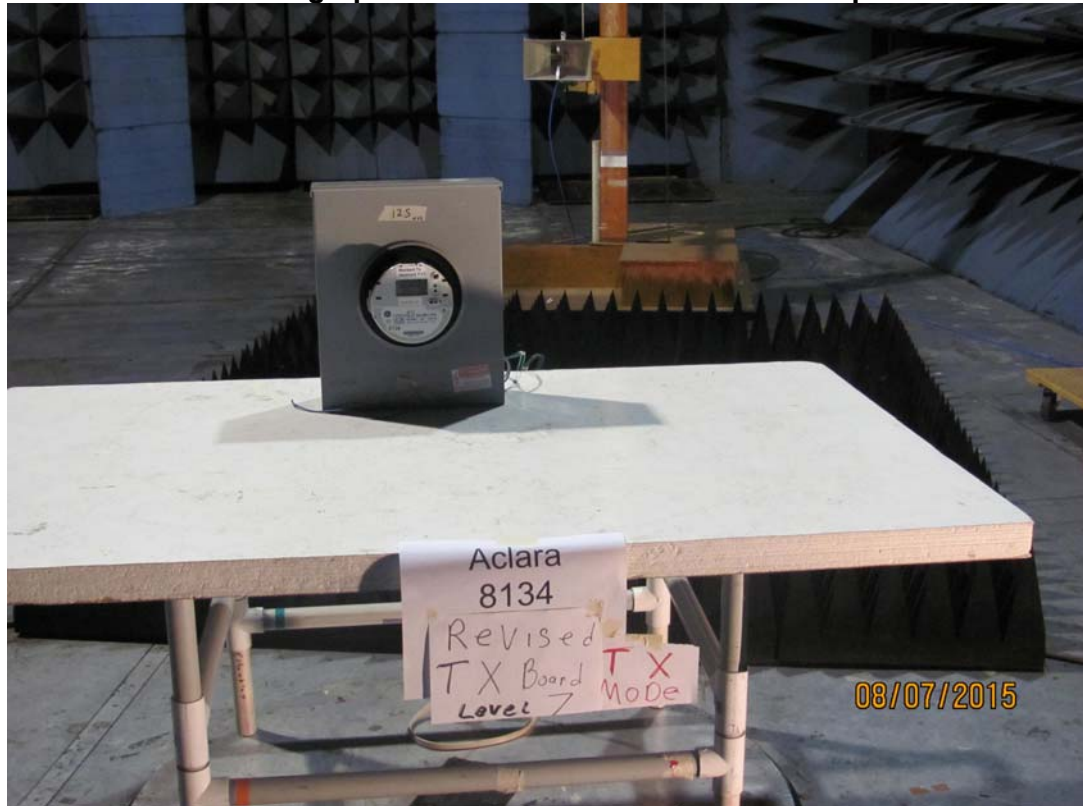
Photograph of Radiated Emissions Test Setup
