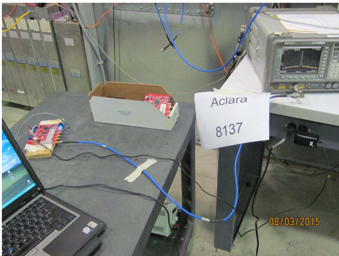
Photograph of Spurious Conducted Emissions Test Setup
