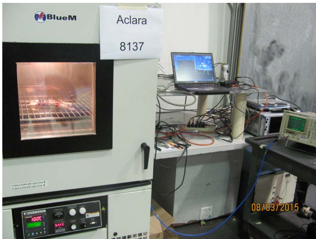
Photograph of Temperature Stability Test Setup
