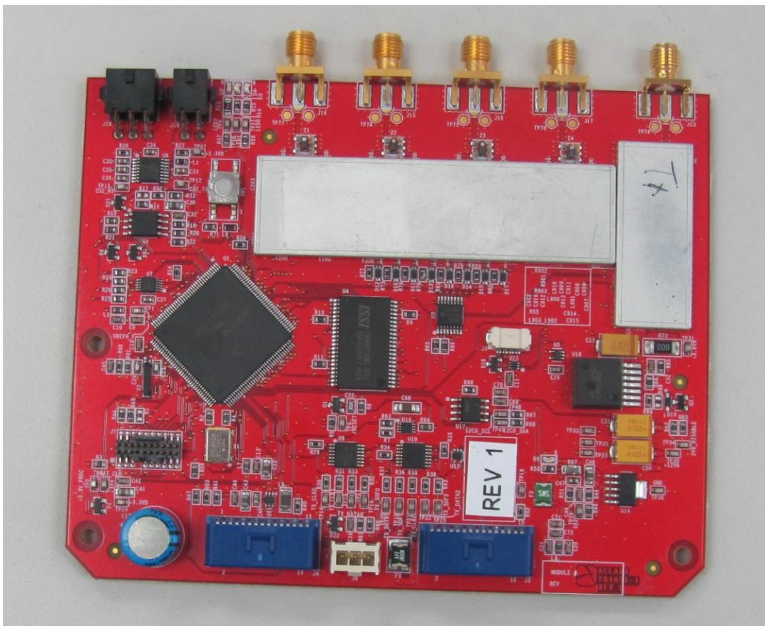
PCB with shields removed
