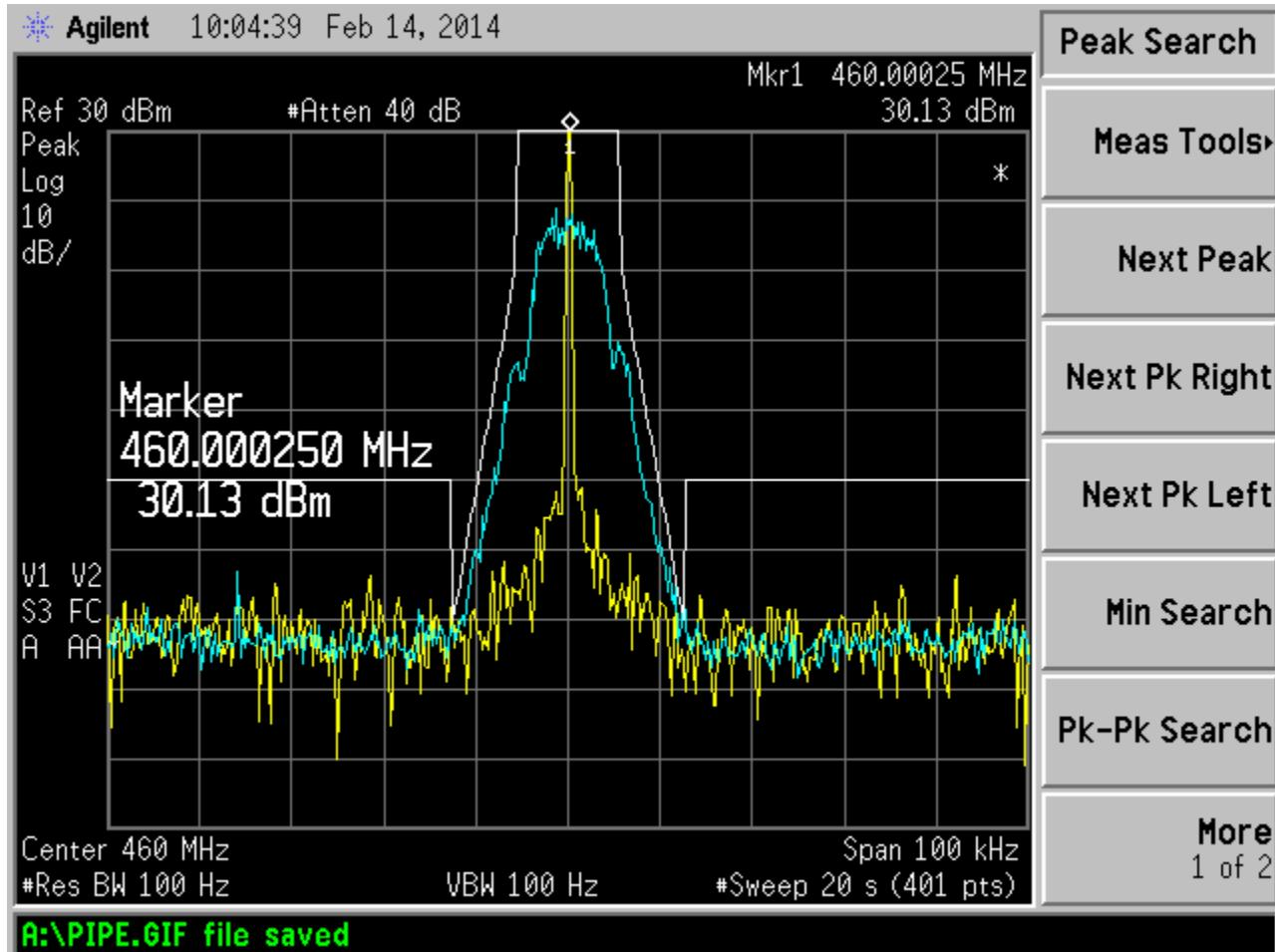
The above plot demonstrates that the EUT meets the 90.210 Emission Mask D requirements:
