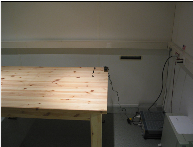
Picture 3 AC conducted emission measurement setup.
