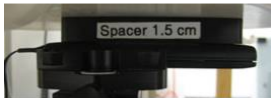
Photo of the device positioned for Body SAR measurement. The spacer was removed for the tests.
