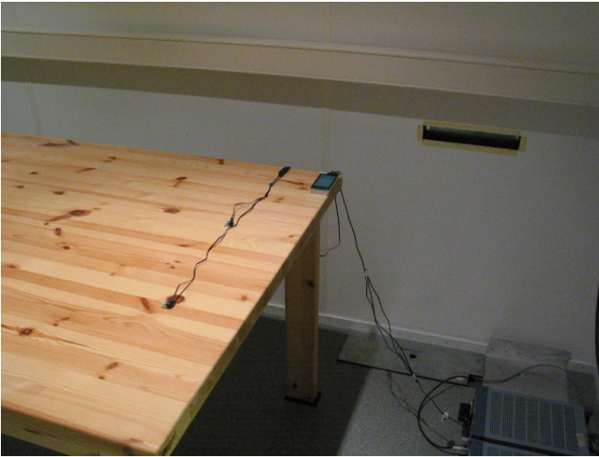
Picture 3 AC powerline conducted emission measurement 15C
