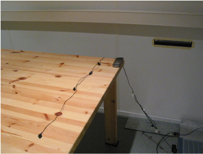
Picture 3 AC powerline conducted emission measurement 15C
