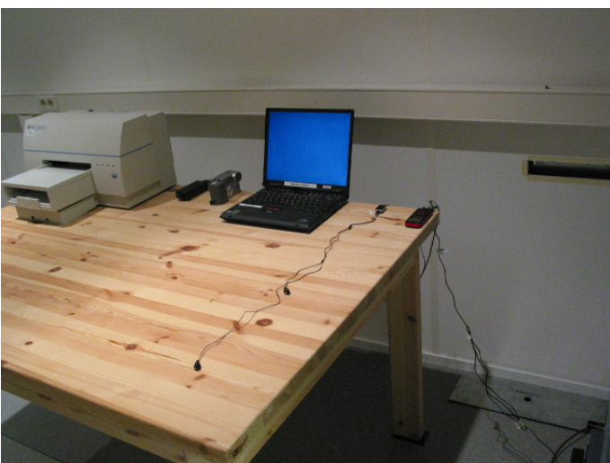
Picture 5 AC powerline conducted emission measurement GSM RX / Bluetooth TX + Computer peripherals
