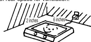
When the air entrance or the air outlet are blocked, the internal temperature of the cooker rises and may automatically shut-off during cooking.
