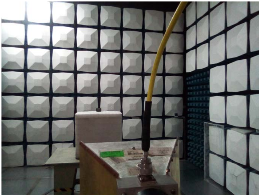
Radiated Emission View (Above 1GHz)
