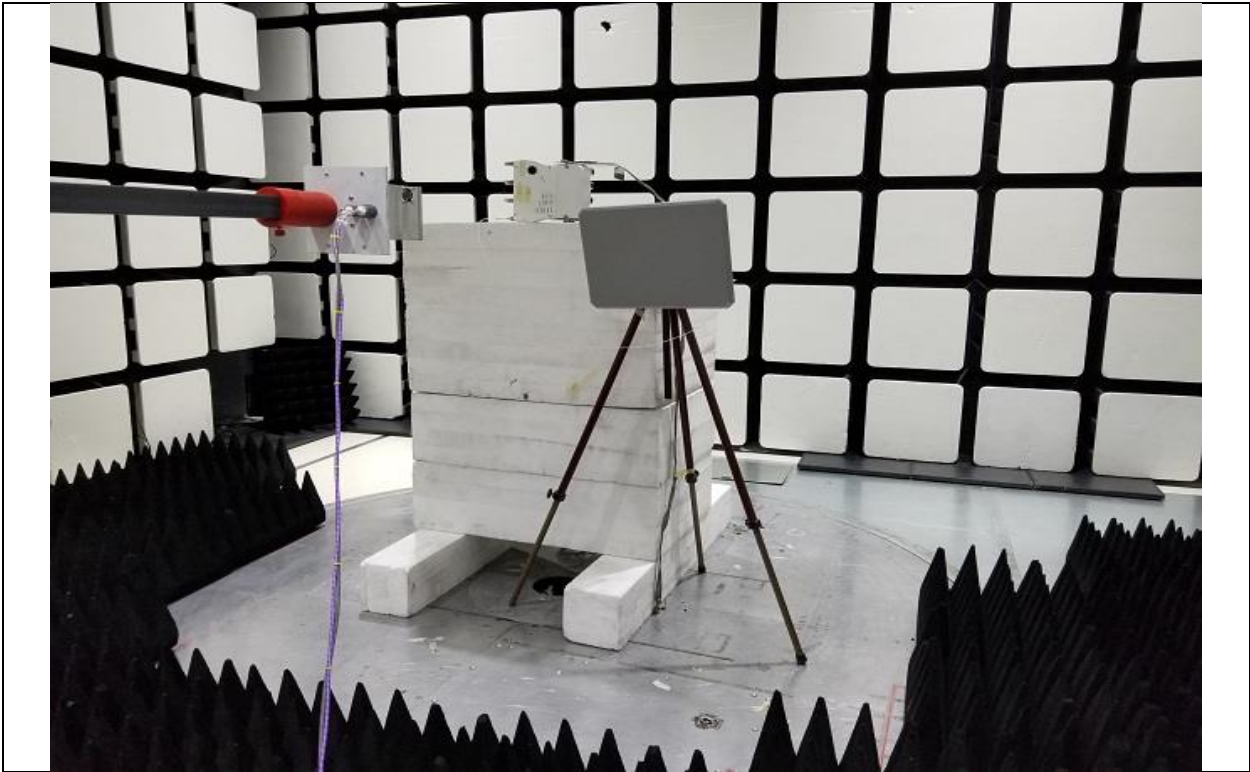
Title: Radiated Spurious Emissions 18GHz-40GHz – Test Setup
