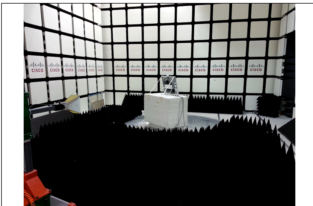
Title: Radiated Spurious Emissions 1G to 18GHz Test Configuration
