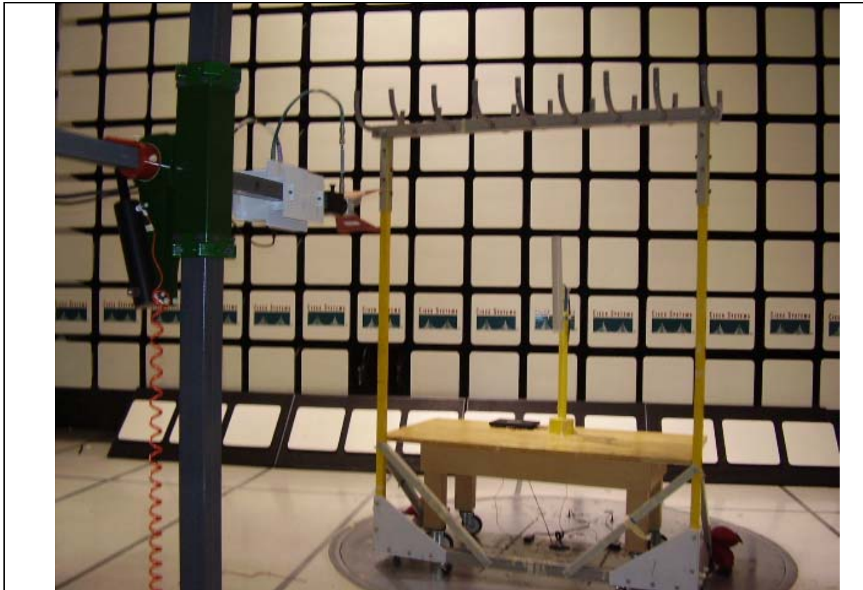
Title: Radiated emissions test setup 17dbi sector
