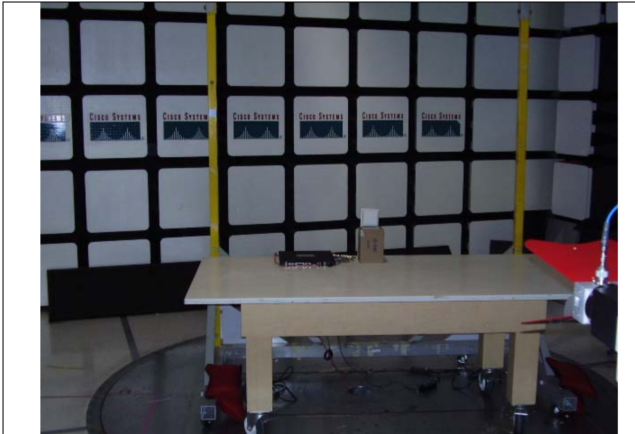
Title: Radiated emissions test setup
