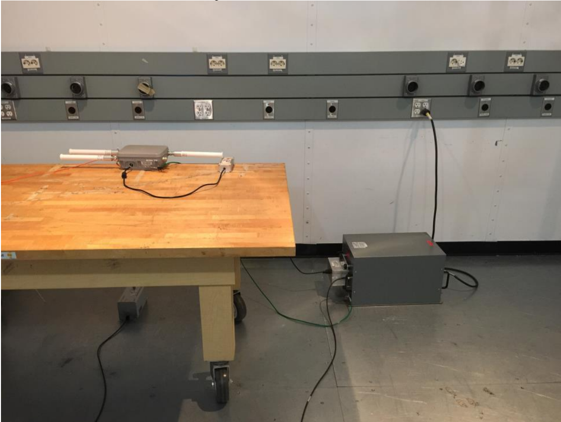
AC Mains Conducted Emissions setup
