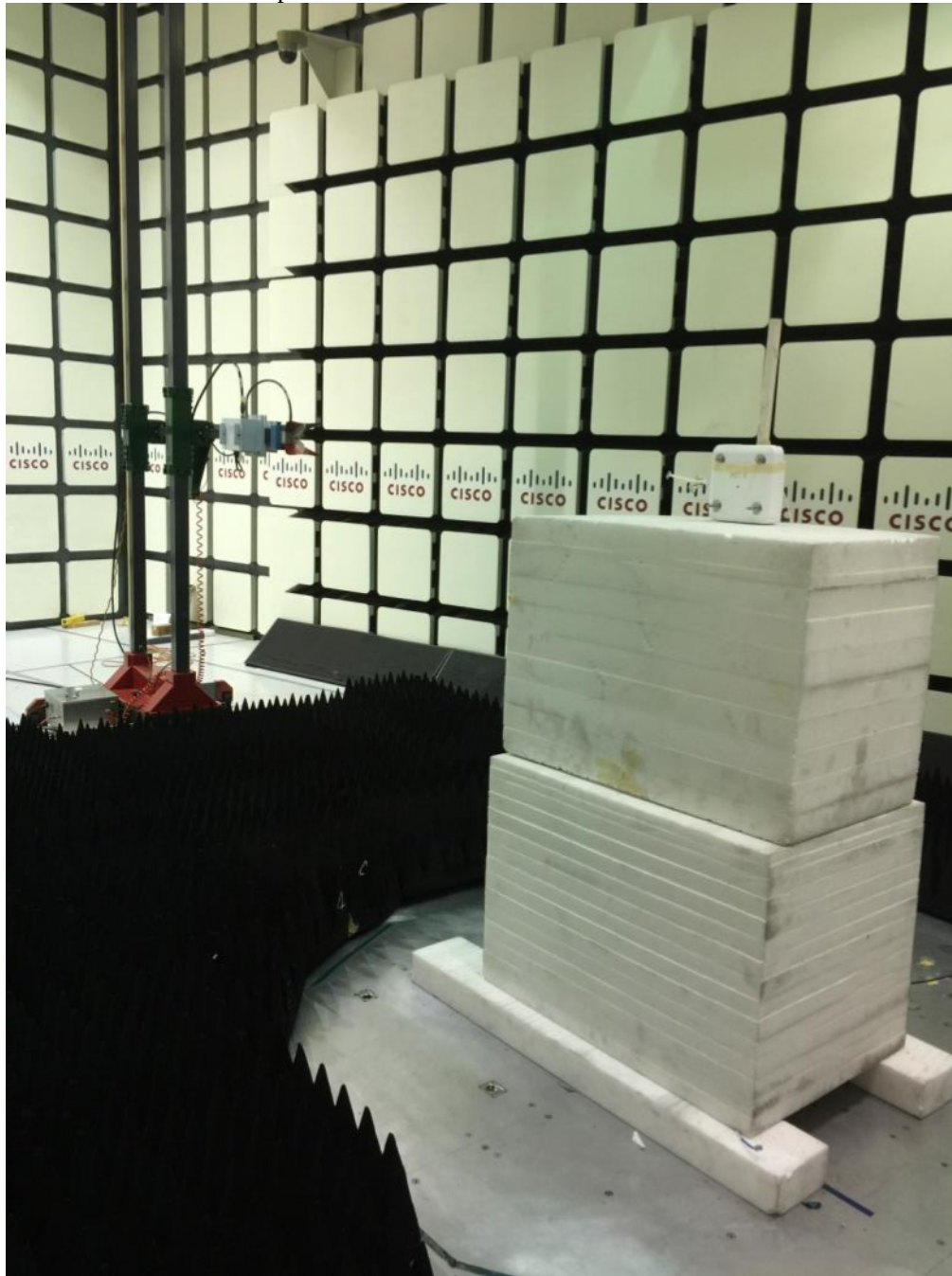
Radiated Emissions setup above 1GHz
