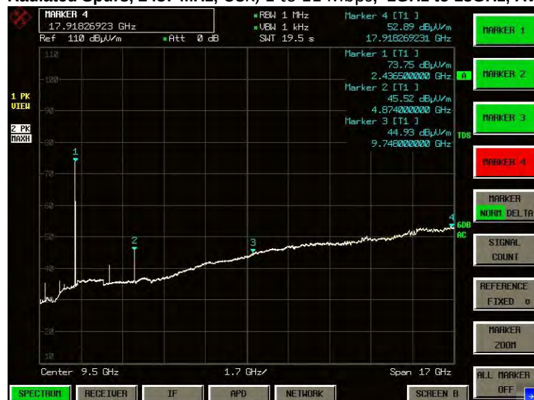
Radiated Spurs, 2437 MHz, CCK, 1 to 11 Mbps, 1GHz to 18GHz, Average plot
