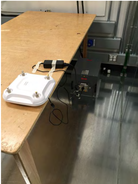
AIR-CAP3702P-B-K9 AC Conducted Emissions setup photo
