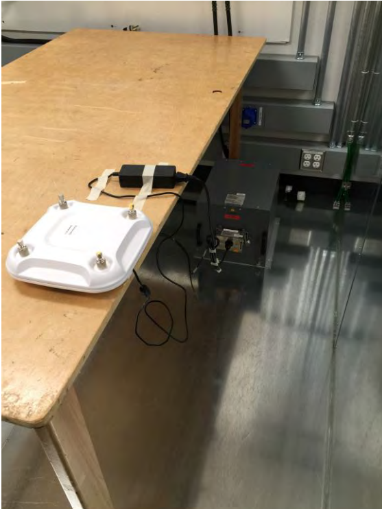
AIR-CAP3702P-B-K9 AC Conducted Emissions setup photo
