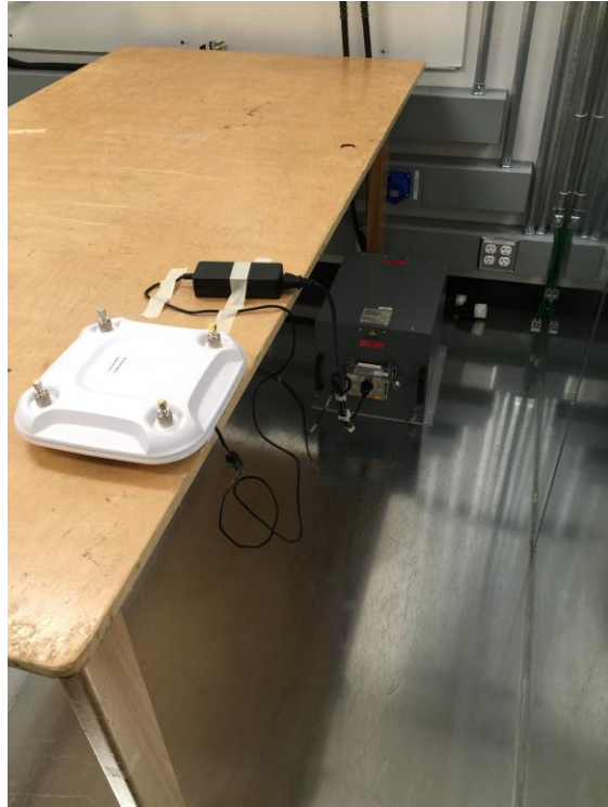
AIR-CAP3702P-B-K9 AC Conducted Emissions setup photo
