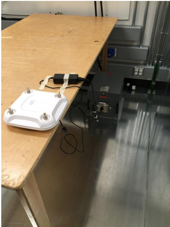
AIR-CAP3702P-B-K9 AC Conducted Emissions setup photo
