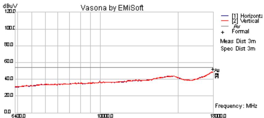
**All Transmit Frequencies, 36Mbps, 6.5dBi Omni-Directional Antenna**
