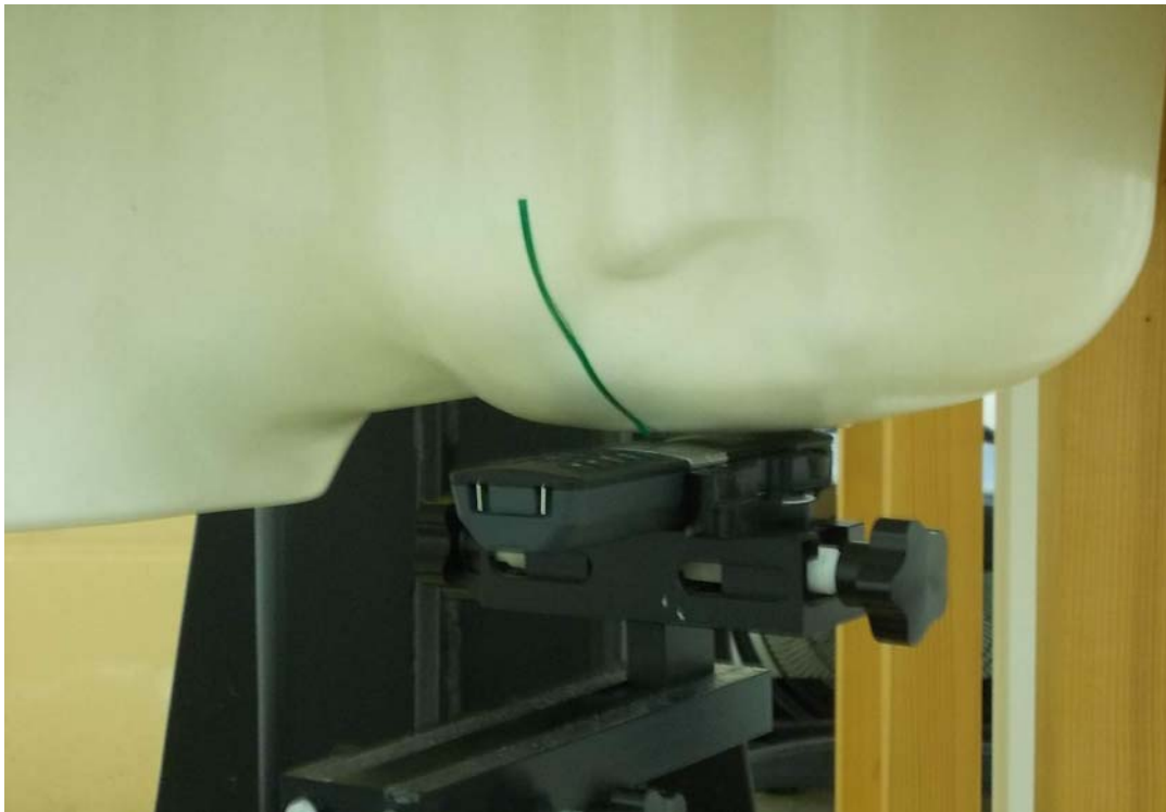
Measurement Position of Left-Cheek (LC) with Handset
