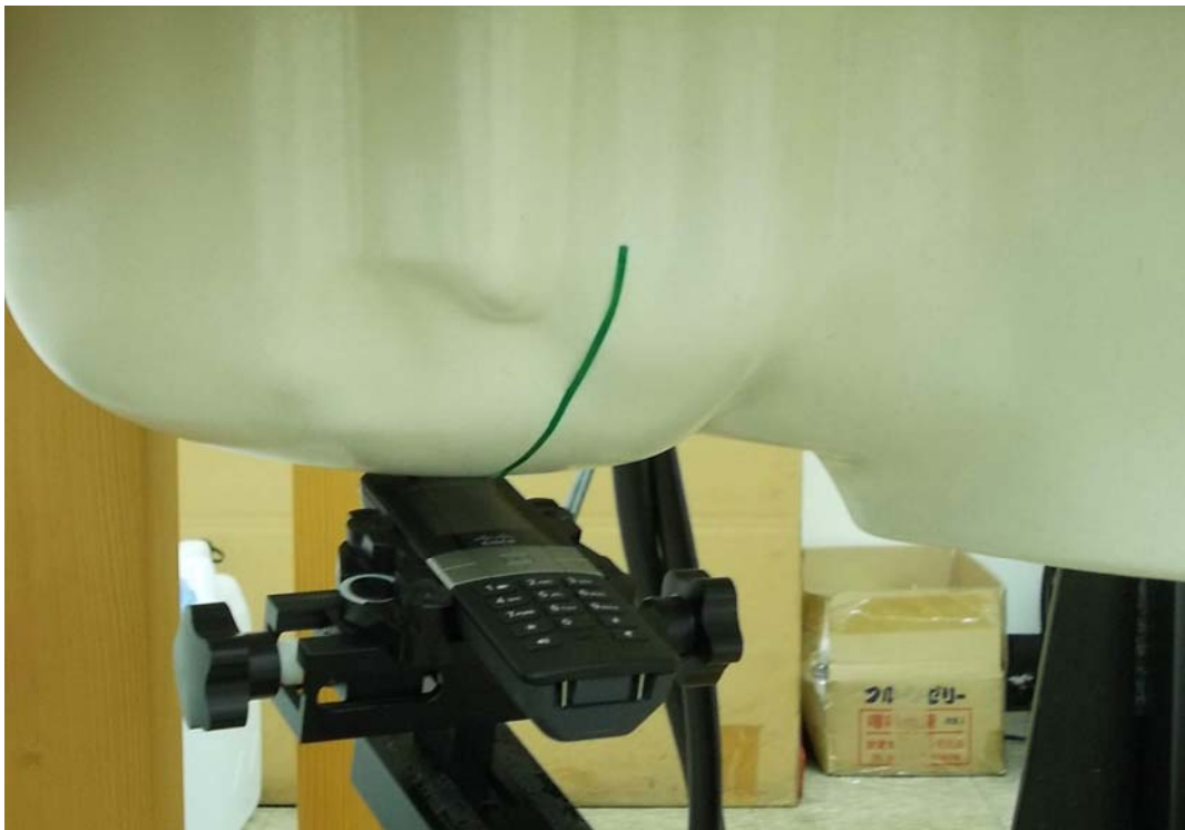
Measurement Position of Right-Tilt (RT) with Handset
