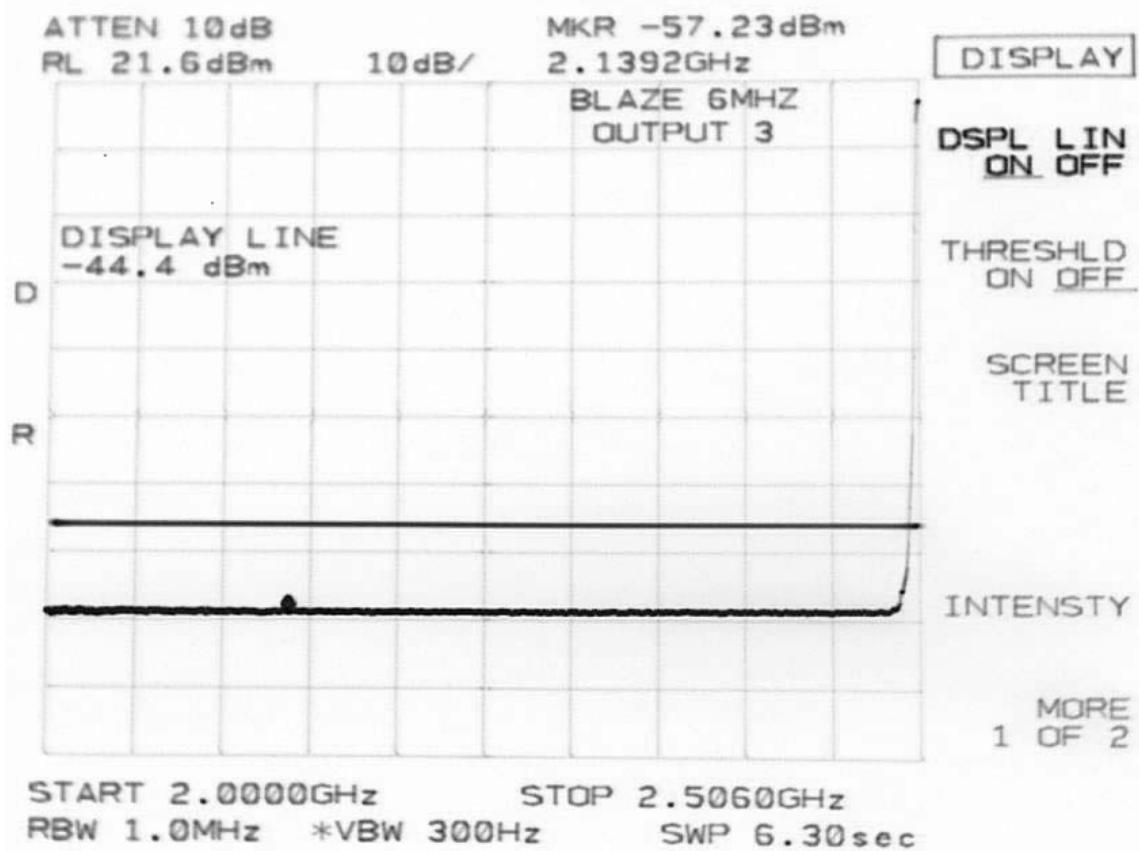
**Antenna Conducted Emissions, 6 MHz Channel Bandwidth (4 of 7)**
