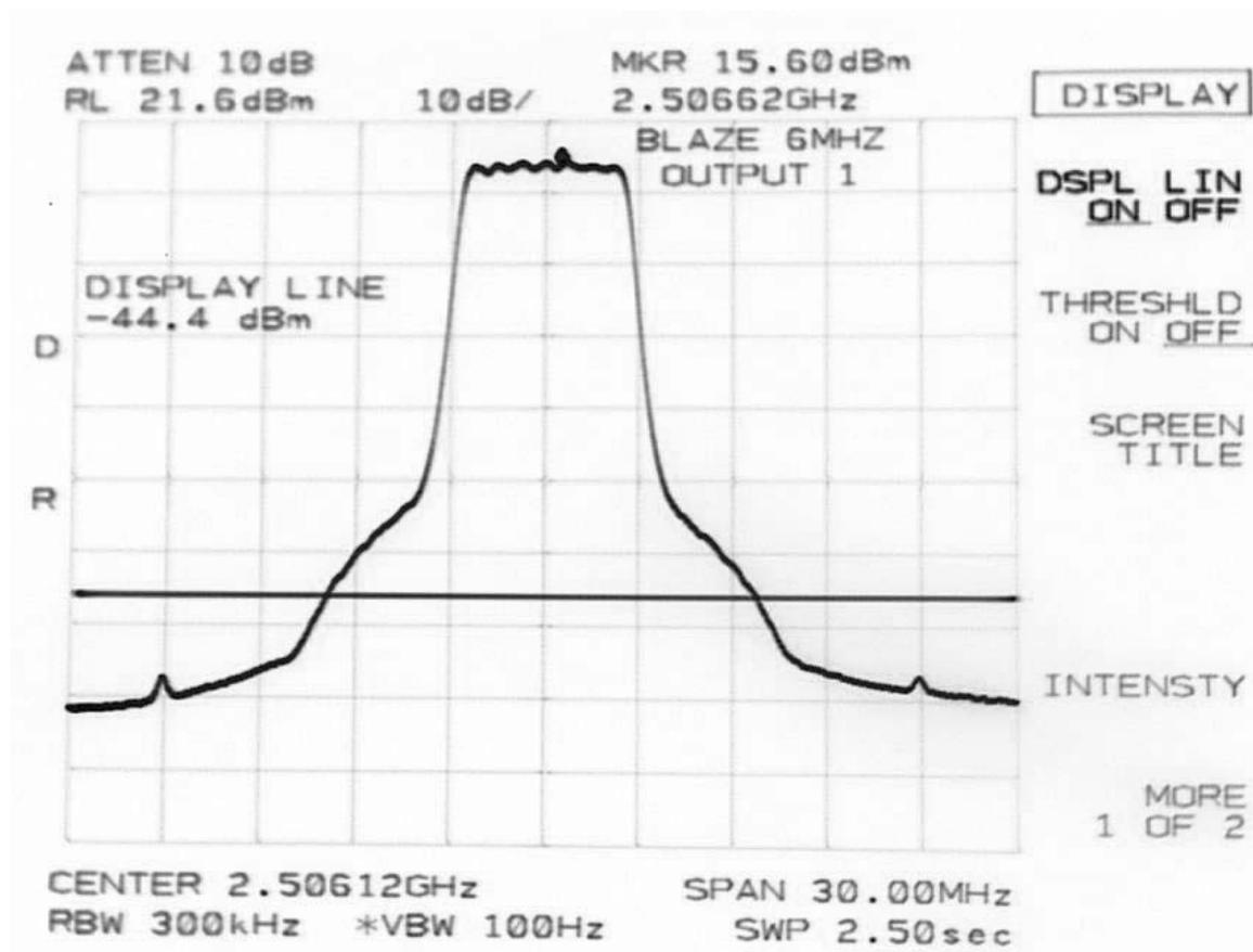
**Antenna Conducted Emissions, 6 MHz Channel Bandwidth (2 of 7)**
