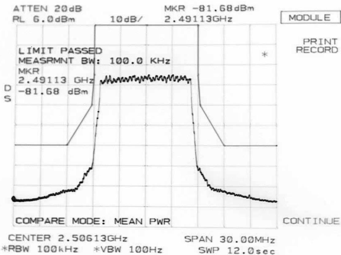
**12 MHz Channel Mask, 100 kHz Peak Power Comparison**
