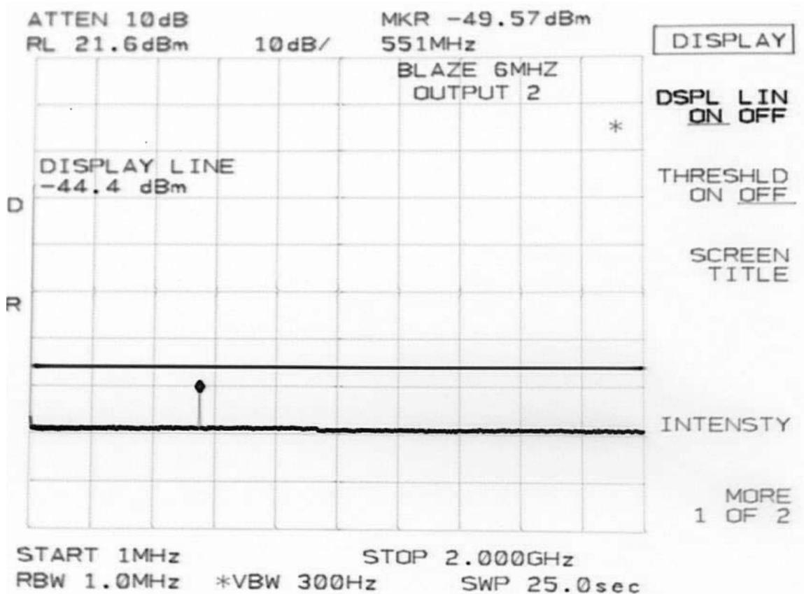
**Antenna Conducted Emissions, 6 MHz Channel Bandwidth (3 of 7)**
