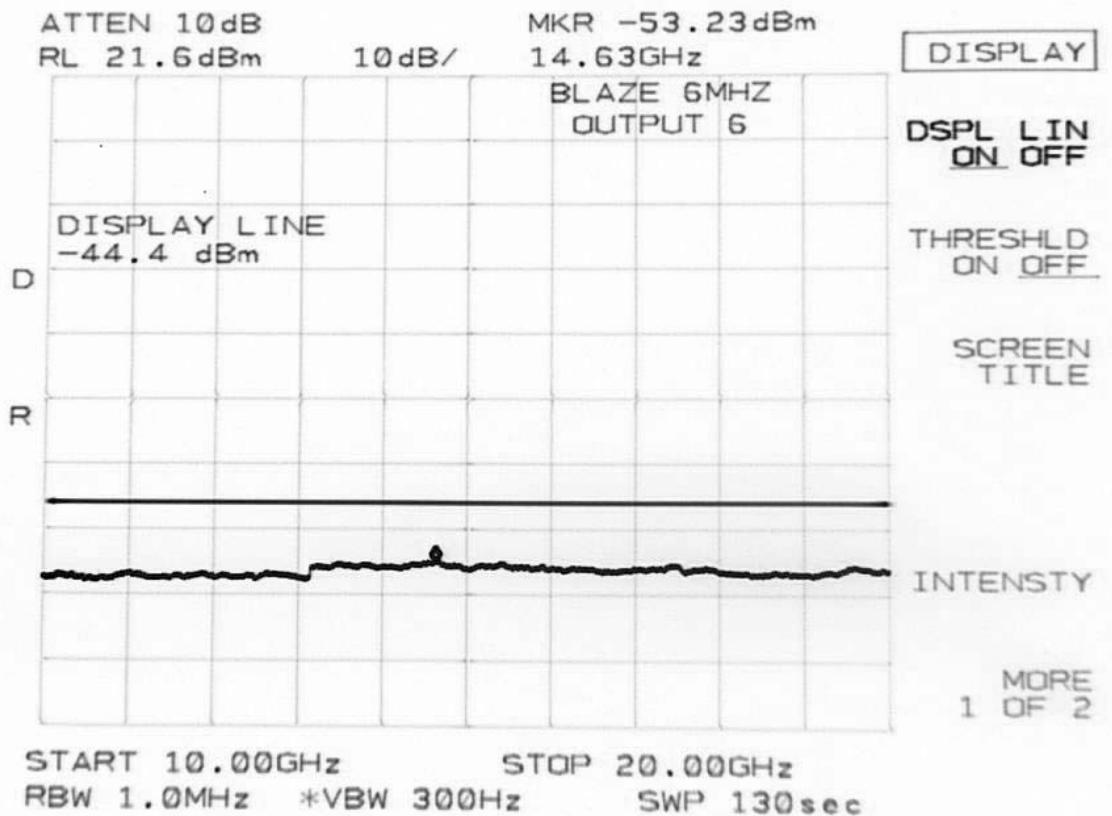
**Antenna Conducted Emissions, 6 MHz Channel Bandwidth (7 of 7)**
