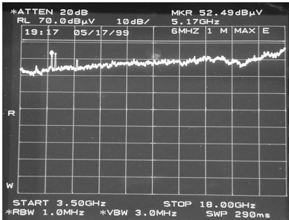
**Case Radiated Emissions, 1 meter Separation**
