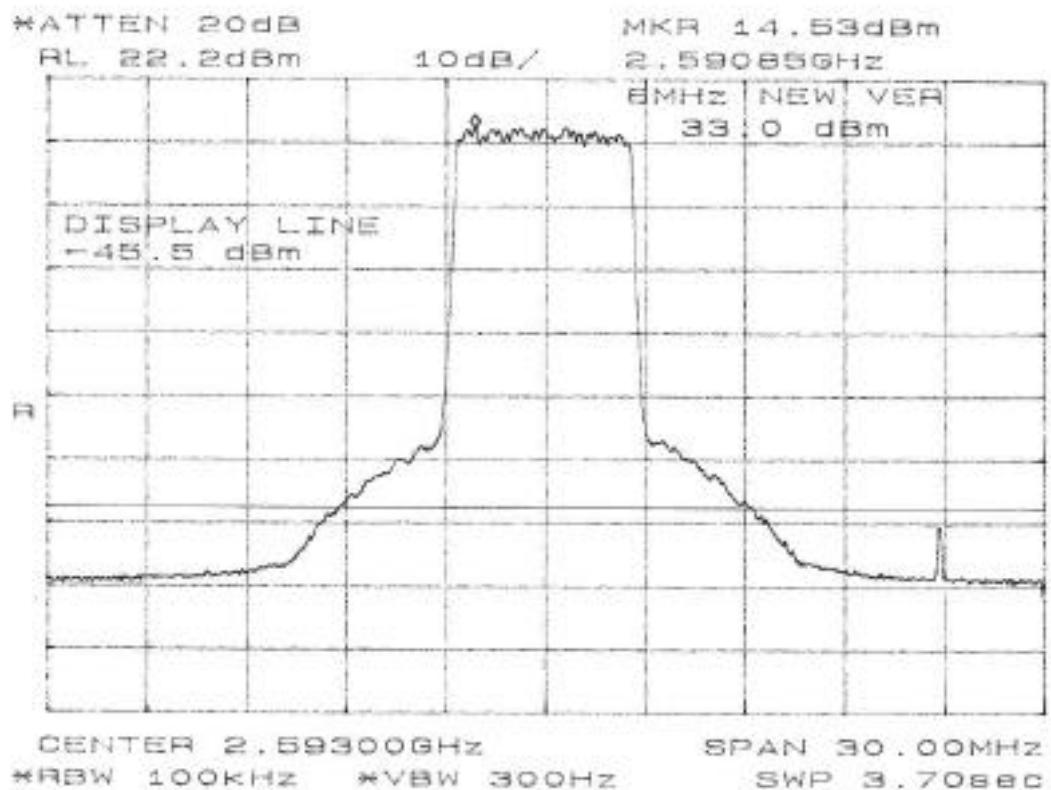
6 MHz TX output, out of band spurious: -48 dBm - 33 dBm output = -81 dBc
