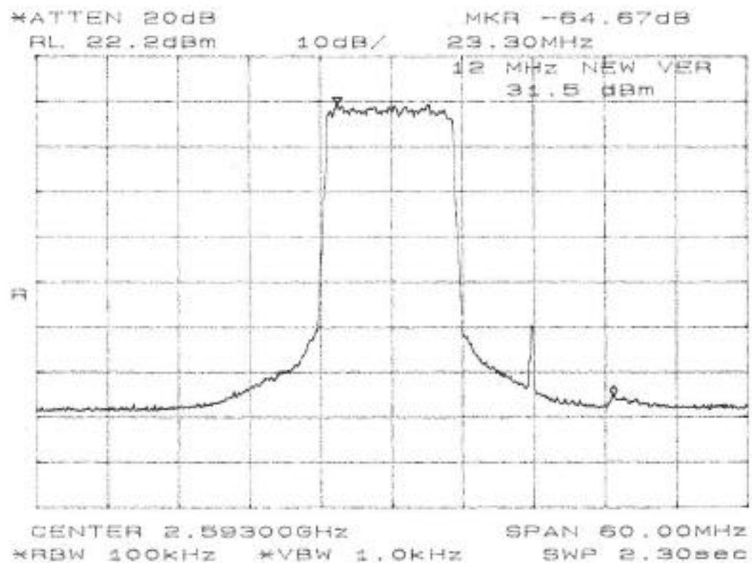
12 MHz TX channel, spurious output: -37.8 dBm - 31.5 dBm = -69.3 dBc
