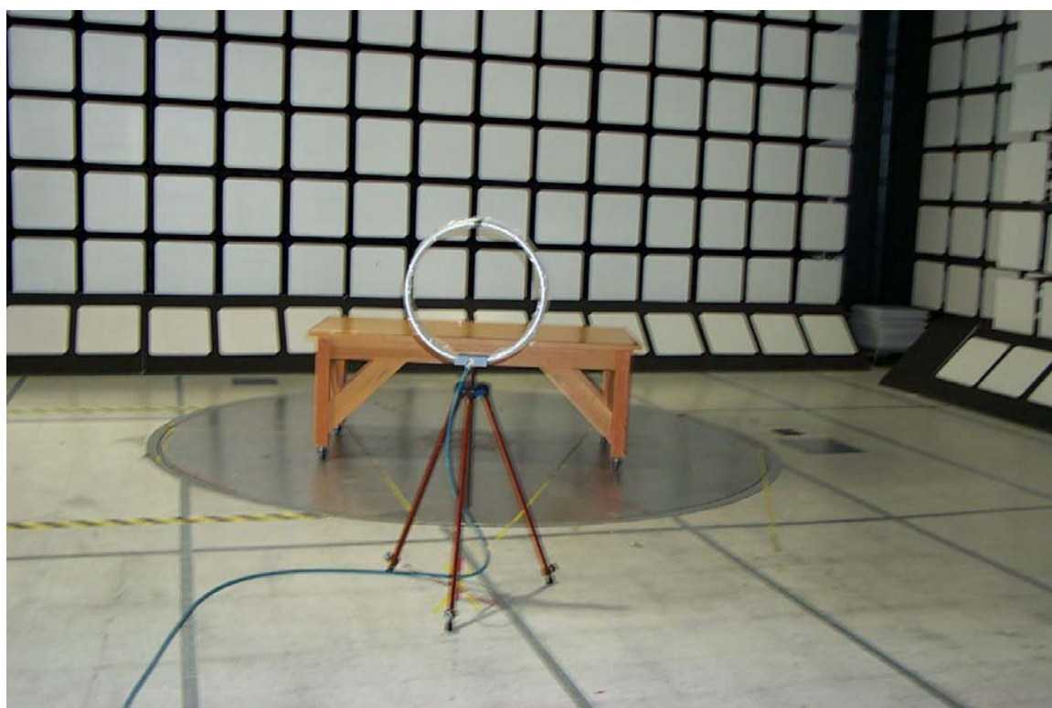
Figure 2 - Test setup, loop antenna at 3m test distance
