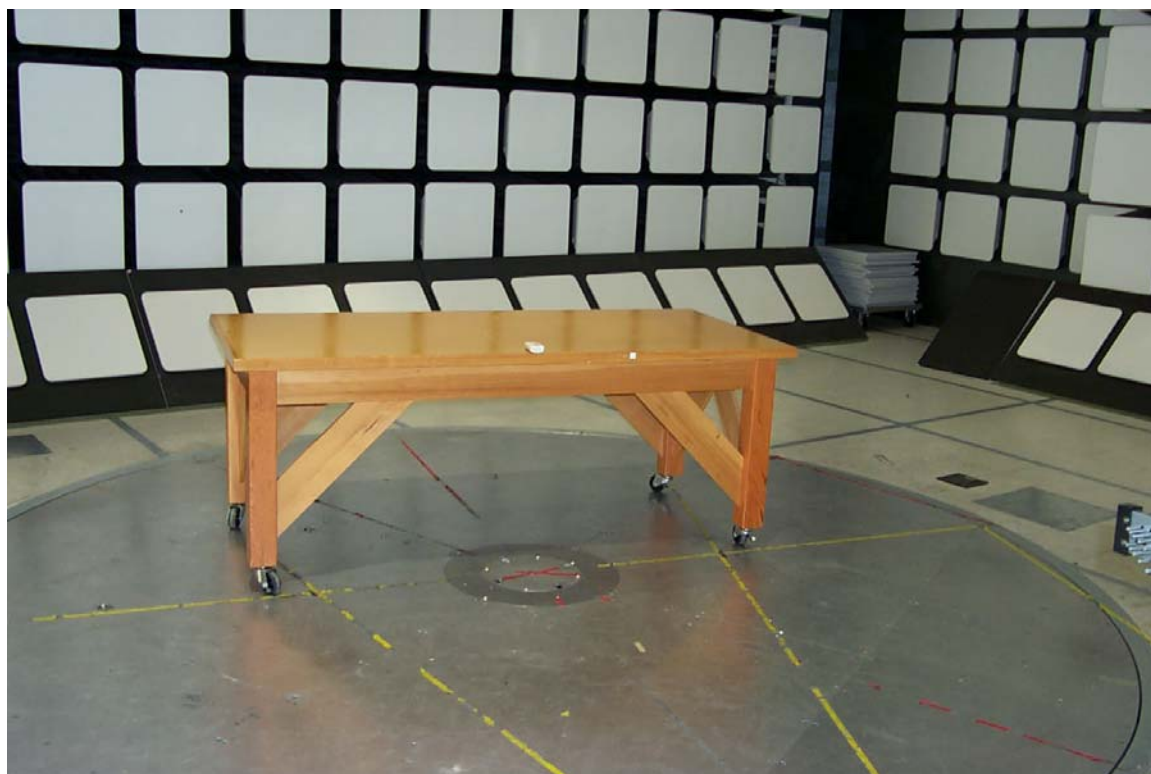
Figure 1 - Radiated Emissions Test Setup
