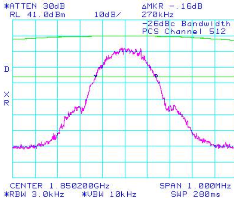
Figure 19: -26dBc bandwidth, PCS1900 Low Channel in GSM mode
