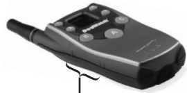
Transmitter Alignment Markers
