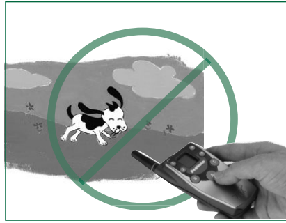
Incorrect Transmitter Position Pointing the transmitter antenna toward your pet will reduce the signal range.
